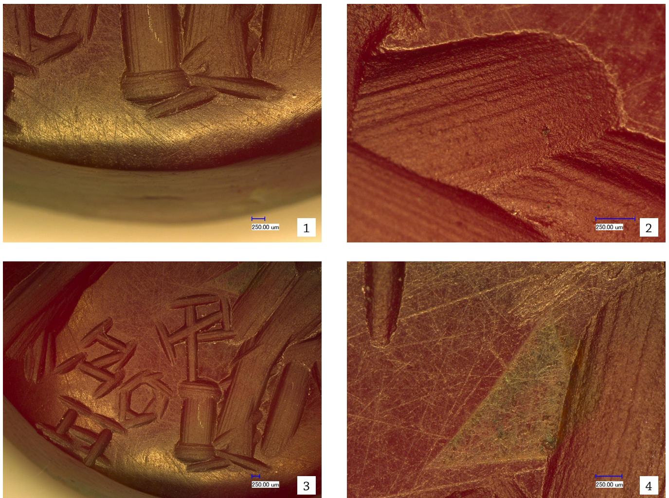
Fig. 8. The gem: technology and engraving details. 1. Polishing striations of the gem 50× magnification; 2. Engraving detail, 150× magnification; 3. Inscription detail, 30× magnification; 4. Gem engraved surface, contact zone with a metal object, 100× magnification (Photos: Dr. M. Mărgărit, 2022; scales are in µm).
